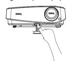
If the projector is not placed on a flat surface or the screen and the projector are not perpendicular to each other, the projected image becomes trapezoidal. To correct this situation, see "Magnifying and searching for details" on page 34 for details.
