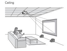
Keep the projector level and place it at a height where its lens is centered between the top and bottom of the screen. If this isn't possible, use the horizontal keystone slider and vertical keystone buttons to adjust the image (see page 24).
