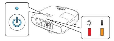
If the projector isn't working correctly, first press the  $\circlearrowleft$  power button, let the projector cool down, and unplug the power cord. Then plug the power cord back in and turn on the projector. If this doesn't solve the problem, check the status lights on top of the projector.
