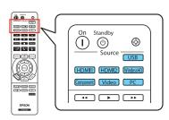
If you press the Source button on the projector, you see a list of available sources. Press the Source button to move through the list and select the desired source.
