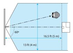
Use the optional external 3D emitter if you cannot view the 3D image normally or if the projector is located more than 16.5 feet (5 m) from the viewing area. See "Optional Accessories" on page 10 for ordering information.
