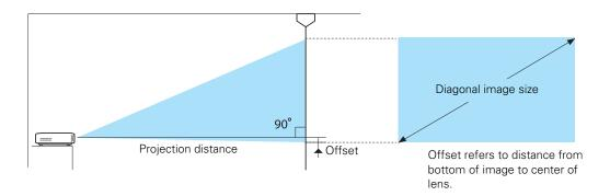
The size of the image is determined by the distance from the projector's lens to the screen. Depending on your display settings and how you use the zoom ring, the actual size may differ. Use these tables as a guide for projector placement:
