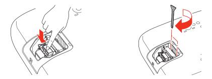
9. Replace the lamp cover. (The projector won't work if the lamp cover is open or loose.)
