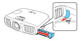
Remove the air filter as shown.
