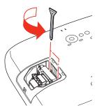
7. Lift up the lamp handle and gently pull the lamp out of the projector.
