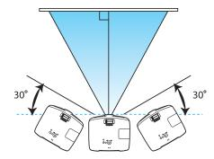
If one side of the image is taller than the other, make sure the projector is parallel to the screen. If necessary, adjust the front feet so that the projector is horizontal.
