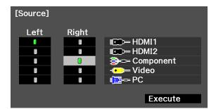
The Left and Right columns represent the left and right screens. Use the arrow buttons on the remote control to highlight Left or Right for the source you want to display. Press Enter on the remote control to select an option.
