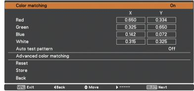
Use the Point ▲▼ buttons to select **Color matching** and then press the SELECT button to display a dialog box. Use the Point ▲▼◀▶ buttons to adjust the setting value.
