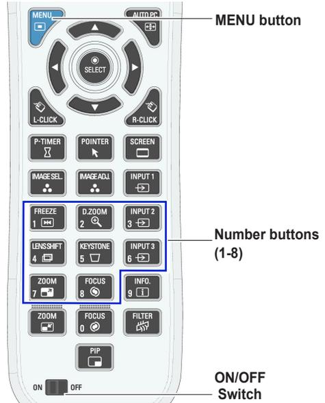
Press and hold the MENU and a number button (1-8) that corresponds to the remote control code for more than five seconds to switch among the codes.
