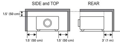
Do not cover the ventilation slots on the projector. Heat build-up can shorten the service life of your projector, and can also be dangerous.
