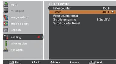
Press the SELECT button to select **Timer** and then use the Point ▲▼ buttons to set the timer. Select from (**Off/400H/700H/1000H**) depending on the operating environment.
