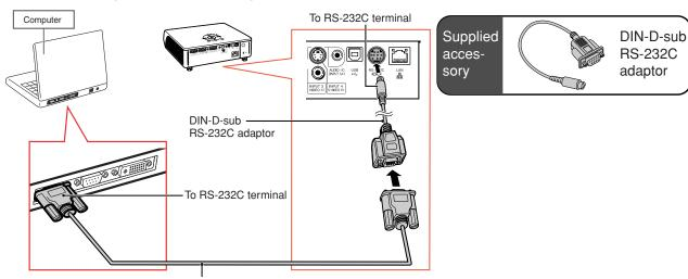
RS-232C serial control cable (cross type, commercially available)
