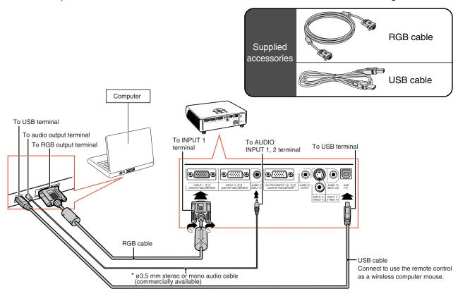
\* When using the ø3.5 mm mono audio cable, the volume level will be half of when using the ø3.5 mm stereo audio cable.
