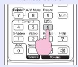
Each time you press the button, the colour mode name is displayed on the screen and the colour mode changes.
