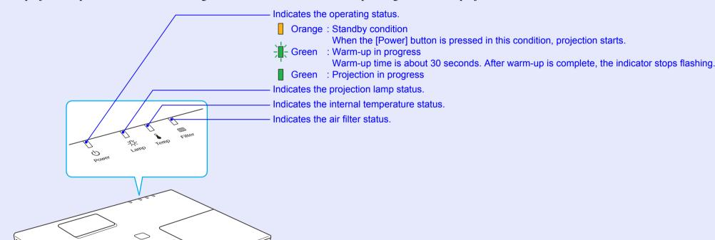
Refer to the following table to see what the indicators mean and how to remedy problems that they indicate. If all indicators are off, check that the power cable is connected correctly and that the power is being supplied normally. Sometimes, when the power cable is unplugged, the  $\circlearrowleft$  indicator remains lit for a short period, this is not a fault.
