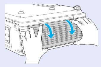
Use a vacuum cleaner to remove dust from the air filter.
