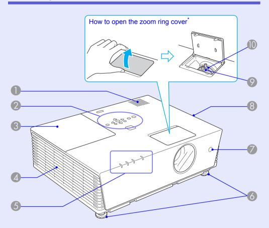
Do not remove the zoom ring cover, and do not use the projector when it is open. Otherwise dust can enter into the projector and shorten the optical engine's service life.
