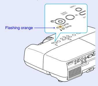
• The projected image gets darker or starts to deteriorate.
