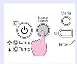
When two or more pieces of equipment are connected, press the [Source Search] button until the target image is projected.
