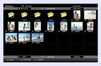
When the projector is connected to multiple storage devices, the following kind of drive selection screen is displayed containing icons that indicate the type of storage. In this case, press the [5] button, and after selecting the drive for the content you want to display, press the [Enter] button.
