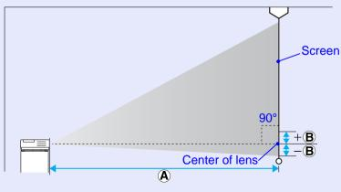
**B** is the distance from the lens center to the bottom of the screen (top of the screen when hung from the ceiling).
