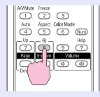
Each time the button is pressed, the area is enlarged. You can enlarge quickly by holding the button down.
