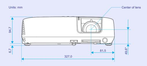
\* Distance from center of lens to suspension bracket fixing point
