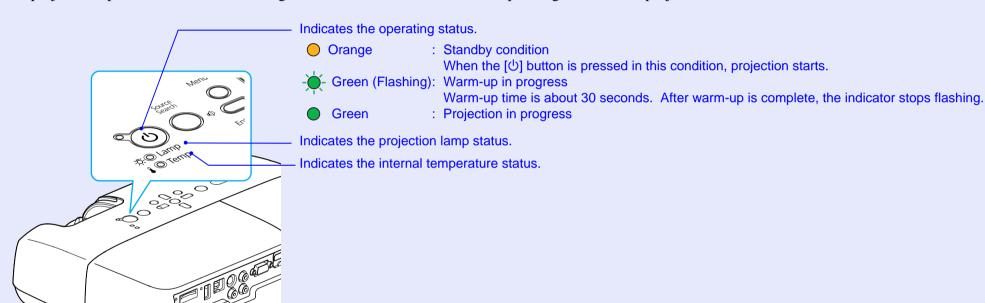
Refer to the following table to see what the indicators mean and how to remedy problems that they indicate. If all indicators are off, check that the power cable is connected correctly and that the power is being supplied normally. Sometimes, when the power cable is unplugged, the  $\circlearrowleft$  indicator remains lit for a short period which is not a fault.
