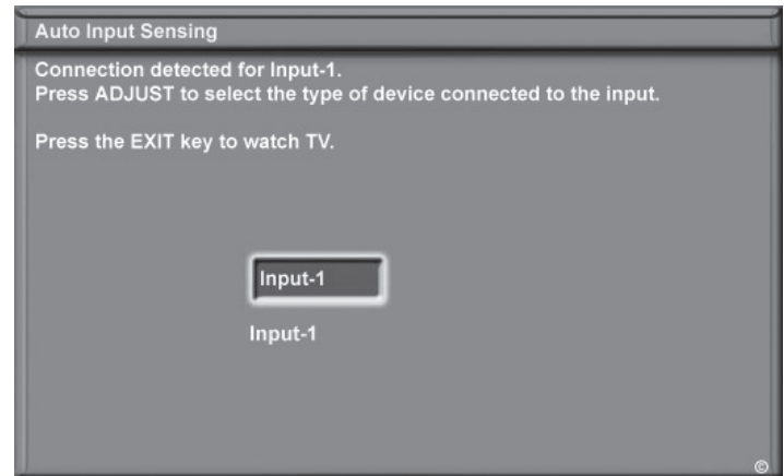
Figure 2. The Auto Input Sensing screen appears when a device is first detected. Select a name for the connected device in this screen.
