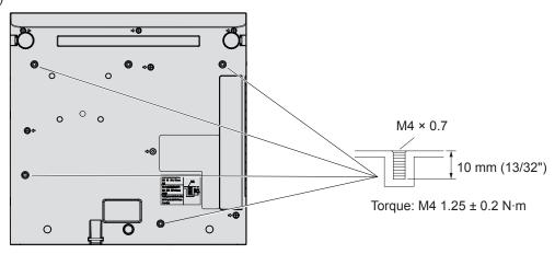
■ Dimensions for the screw holes to fix the projector (projector bottom view) Unit: mm (inch)
