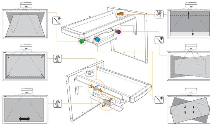
Use the mechanical adjustments described in the installation document and the image alignment screen to adjust the projected image size, shape and location so that you can see the full projected image clearly. Don't use other images, which might be cropped or scaled by the projector and result in a misleading projected image size, shape and location.
