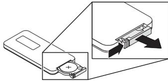
2. Remove the old battery from the battery holder and replace it with a CR2025 coin-cell battery.
