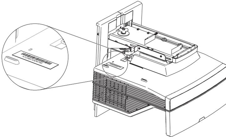
The serial number is also located at the bottom of the projector and can be seen when you stand on the floor and look up at the projector. Open the cable cover at the bottom of the projector and locate the serial number next to the cable connectors.
