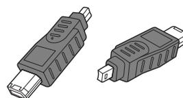
Connecting a 6-pin device (such as a camcorder) directly to the TV, (if it is designed to receive electrical power from another 6-pin device) will require that the camcorder is directly connected to the AC supply, or that the camcorder's battery power is used.
