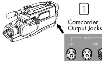
**2** Connect a set of audio cables between the AUDIO IN jacks on the TV and the AUDIO OUT jacks on the camcorder. If you have a mono Camcorder, connect L(mono) to the Camcorder audio out using only one audio cable.
