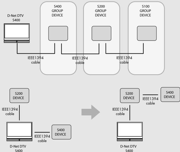
※ A 1394 device has a maximum connection speed which will be marked near the IEEE 1394 connector with an "S" number (i.e., S100,S200,S400). The higher the number, the faster the maximum connection speed. This TV has a maximum connection speed of S400.
