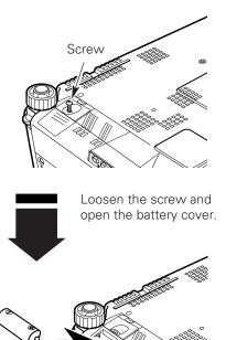
Install the battery then replace the battery cover and secure it with the screw.
