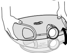
② Adjust the angle and direction of the projected image as you want by lifting up the projector and rotating the projector on the Swivel Stand.
