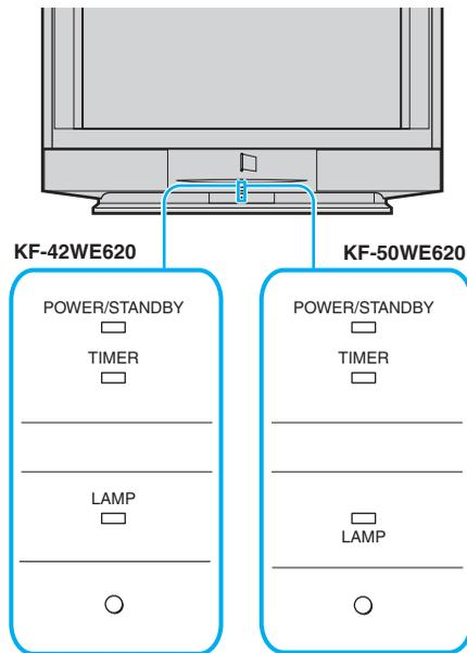
The POWER/STANDBY (red) and/or LAMP (red) indicators show the conditions of the LCD projection TV and warnings by lighting or flashing, as follows.
