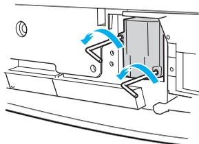
Loosen the two screws with the hex key supplied with the lamp.
