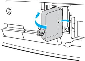
Align the right side of the lamp cover with the hole on the unit, and replace the lamp cover in its original position.
