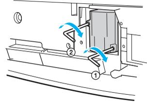
Tighten the two screws securely first ①, then ② with the supplied hex key, as shown in the illustration.
