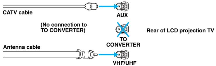
Select CABLE or antenna (ANT) mode by pressing ANT on the remote control.
