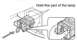
**8** Put the new lamp into its place. For KS-60R200A/50R200A, slide it in slowly by pressing the PUSH part of the front corners of the lamp until it stops with a firm clicking sound to lock. For KS-70R200A, make sure the lamp is
