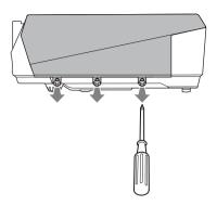
**3** Remove the lamp cover by lifting it forward with the fingers placed on the slit of the projector.
