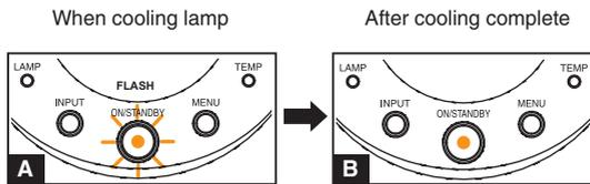
**A** During cooling, the ON/STANDBY indicator flashes. In this state, the power cannot be turned back on. However, there is no problem with unplugging the power cord in this state.
