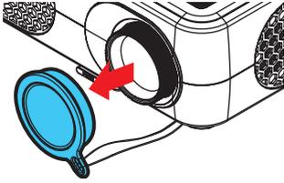
Be sure to remove the lens cover when the power is turned on. If the cover is left on the projector, it could become deformed due to heat.
