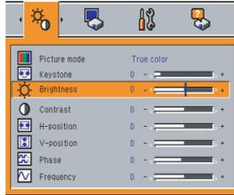
Displays the current adjustments and settings of selected category. Item shown with gray cannot be adjusted with the current input source.
