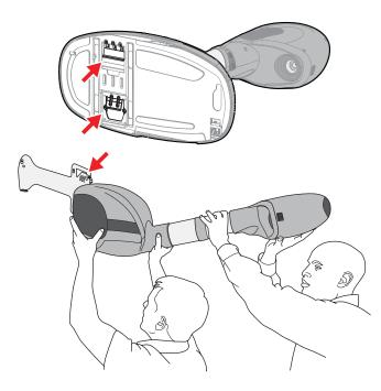
9. Using 2 people, slightly push up on the unit to make sure unit is locked on mounting plate
