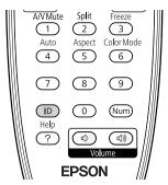
While holding the ID button, press a numbered button on the remote control (0 through 9) to select the desired ID. Select zero to control all projectors, or select a number to match the ID of the projector(s) you want to operate.
