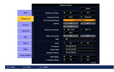
4. Select **To Setup Wizard**, then press **Enter**. You see the WPS (Wi-Fi Protected Setup) connection screen:
