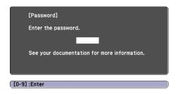
Hold down the Num button on the remote control and use the numeric keypad to enter the four digit password. The password screen closes and projection begins.
