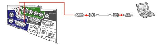
4. Tighten the screws on the VGA connectors.
