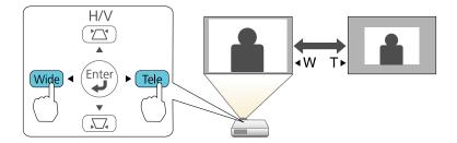
**Note:** If the projector is installed out of reach, you can also adjust the image size using the Zoom setting in the projector menus.
