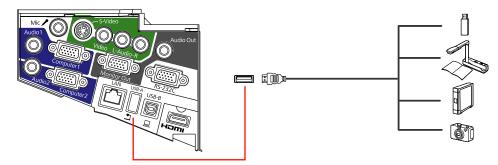
**Note:** Do not connect a USB hub or a USB cable longer than 10 feet (3 m), or the device may not operate correctly.
