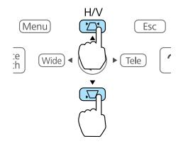
3. Press a keystone button on the projector's control panel to adjust the image shape.
