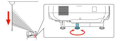
4. If the image is tilted, rotate the rear feet to adjust their height.
