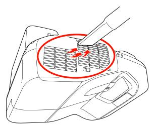
**Note:** You can remove the air filter so you can clean both sides of it. Do not rinse the air filter in water, or use any detergent or solvent to clean it.
