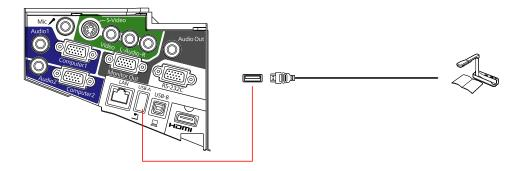
3. Connect the other end of the cable to the document camera's USB Type B port.
