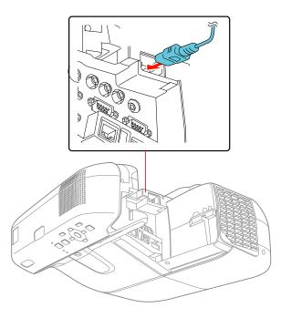
2. Plug the power cord into an electrical outlet.
